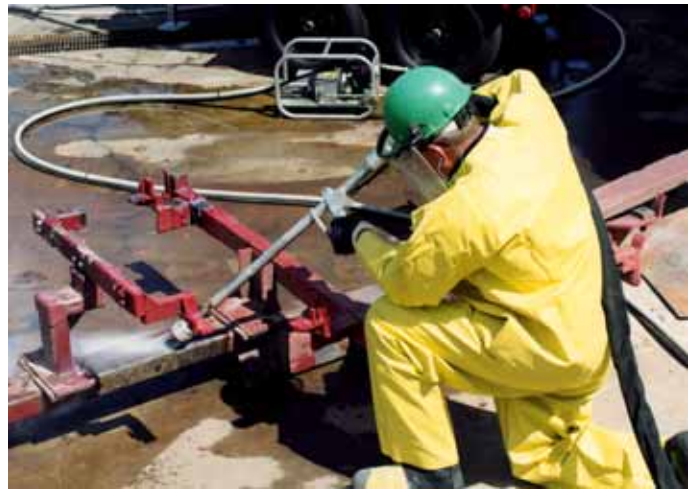
Paint removal for automotive skids using the NLB Model NCG8400A-3 rotating hand lance.
