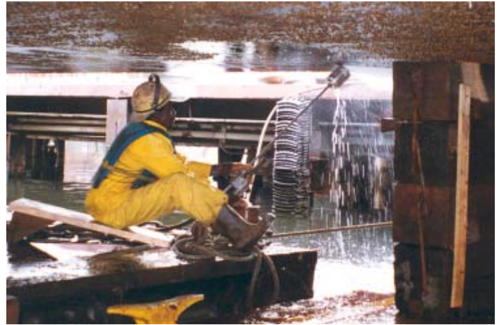
The 17 gpm at 15,000 psi is applied to the hull with an NLB 20-282 hand lance and a model SRH 20-77 SPIN-NOZZLE.
