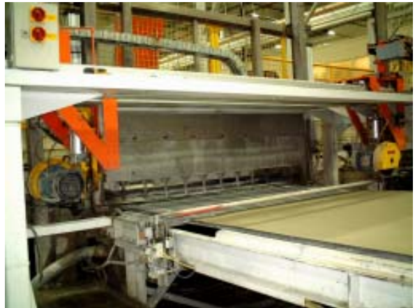
An uncut sheet of siding material prior to passing under the waterjets.
