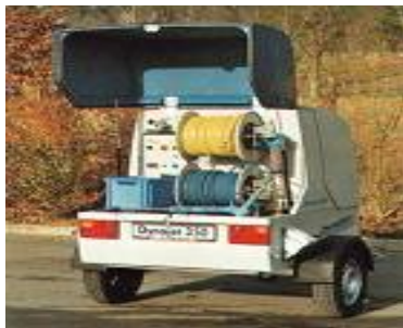
The TARGA design feature gives a practical separation of work area (blue hood) and engine compartment (grey hood)
