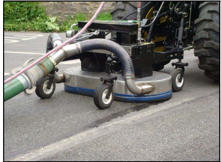
Twin NLB 24\"UHP Spinjets Hydraulic Driven from a Single Hydraulic Motor C/w Full Vacuum Recovery
