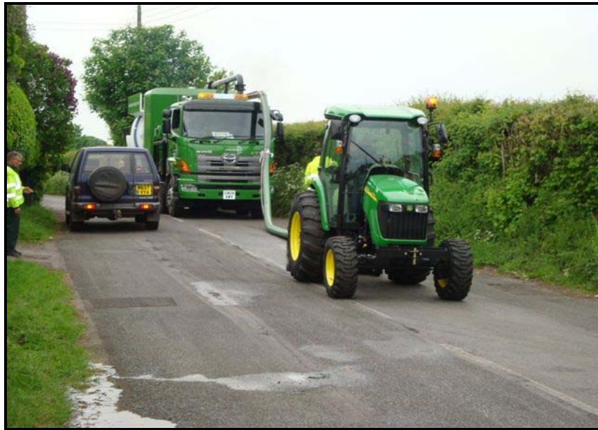
Mini Tractor c/w Hydrostatic Drive & Rear Mounted Twin NLB 24\"UHP Spinjets
