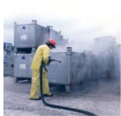
The 6 gpm (22.7 lpm) at 36,000 psi (2,500 bar) is easily applied with the NLB model 8400A rotating lance.
