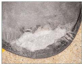
Only first layer had any penetration.
