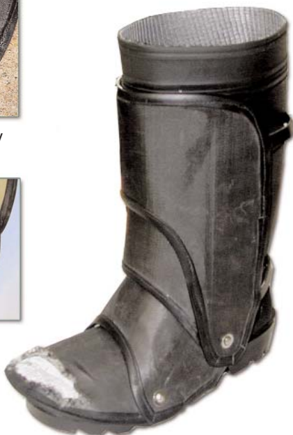
Only first layer had any penetration.
